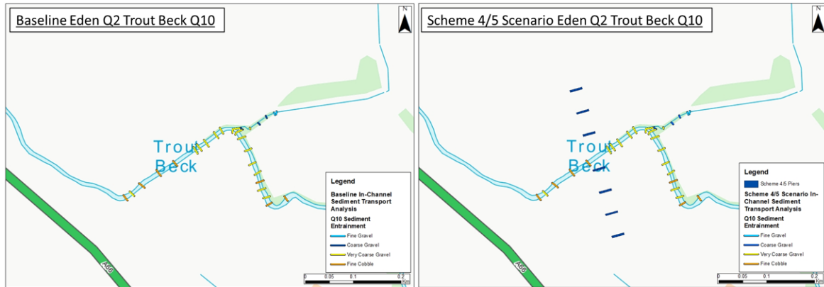
Plate 1-6: Comparison of hydraulically modelled sediment entrainment size for the River Eden 1-in-2 Year and Trout Beck 1-in-10 Year Flood Event
